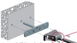
recommended fixing panhead screw M5x12 mm
