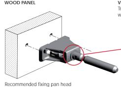
VERY IMPORTANT Triade Maxi has to be installed with the arrow facing upwards.
