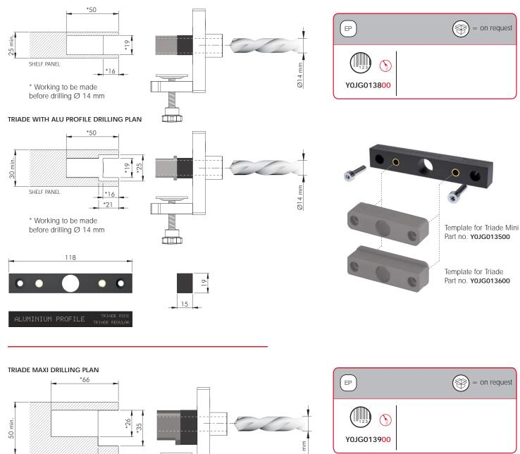
\* Working to be made before drilling Ø 14 mm
