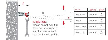
SCREW THE LOCKING BOLT TO BLOCK THE PIN
