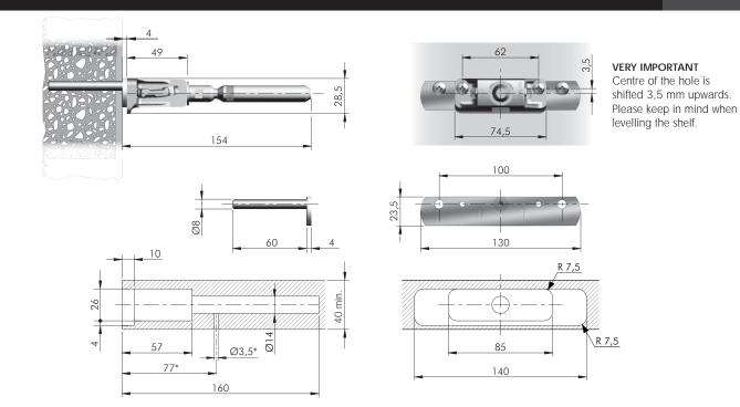
\* Optional drilling for security locking with M4 grub screw placed underneath in alignment with the cavity. For details refer to Triade Maxi section.
